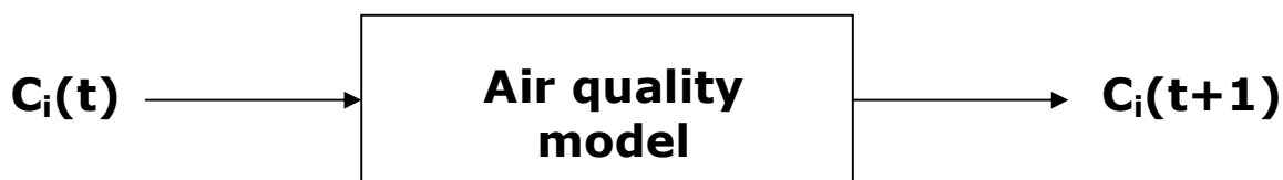
Figure 1.1. Air quality model calculates the evolution of concentration fields of air pollutants, in subsequent timesteps ( C_i – concentration of “i” modelled species).
